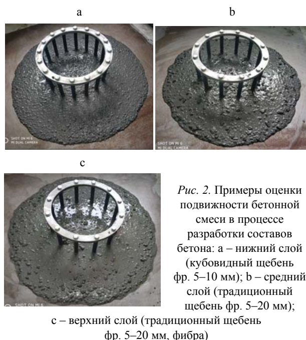
Fig. 2. Examples of assessing mobility of concrete mixture in the process of developing concrete compositions: а – bottom layer (cuboid crushed stone fraction 5–10 mm); б – middle layer (traditional crushed stone fraction 5–20 mm); в – top layer (traditional crushed stone fraction 5–20 mm, fiber)
