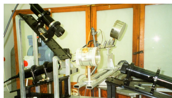
Fig. 5. Test chamber for testing the atomization and combustion process
