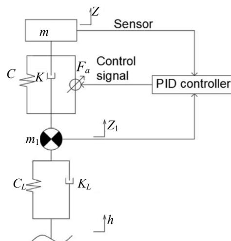
Fig. 1. Dynamic Diagram of the active suspension system
