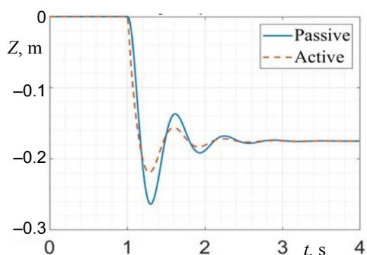
Fig. 10. Vehicle body displacement
