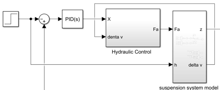
Fig. 3. Simulation model structures of an active suspension system
