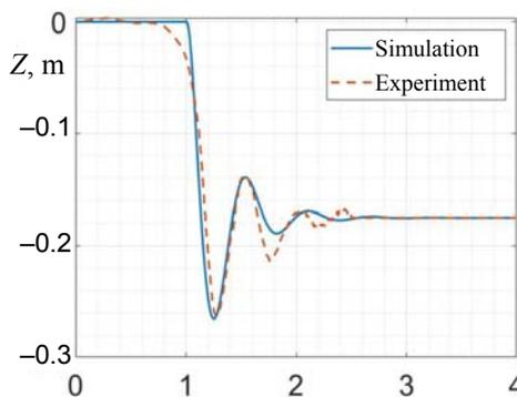
Fig. 8. Comparison of simulated and experimental displacement of the sprung mass in the passive suspension system
