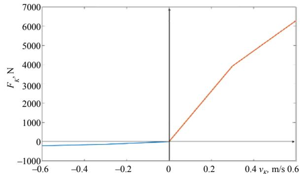
Fig. 7. Equivalent damping characteristics as input for simulation
