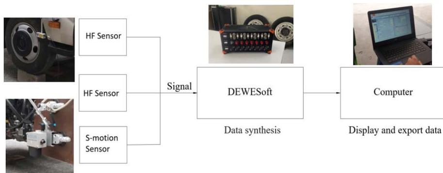
Fig. 5. Experimental configuration for determining the vehicle vibration
