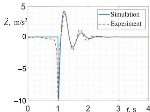
Fig. 9. Comparison of simulated and experimental vehicle body acceleration in the passive suspension system
